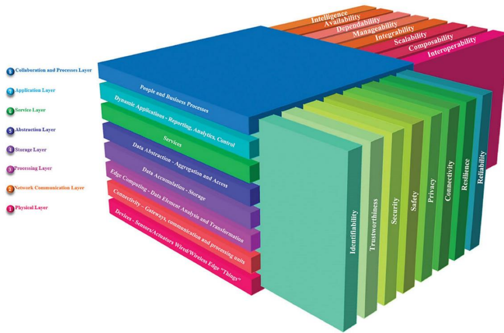
Figure 45: The general structure of CREATE-IoT 3D RAM 953
